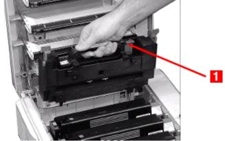
7. Push the two blue retaining levers (1) toward the rear of the printer to lock the fuser in place.
